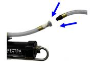
\*Connecting brine discharge service hose at quick disconnect
