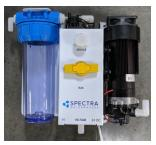
\*Service valve OFF, in FLUSH position
