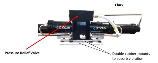
**NOTE:** This module **must** be installed in an area that maintains a temperature below 113°F (45°C). It may be placed as high in the boat as you desire, and mounted in any position, even upside down. Make sure that the area around and under the pump does not have any water sensitive equipment, as water will be spilled during any repairs or if a leak occurs. Allow for easy access to the pressure relief valve.
