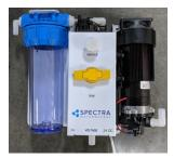
Service valve OFF, in FLUSH position
