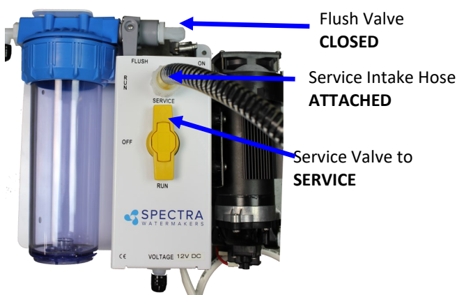
Valves in SERVICE position:
