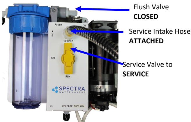
Valves in SERVICE position:
