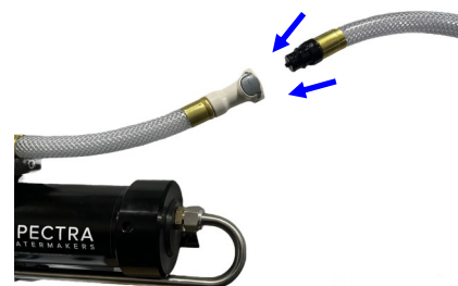
Connecting brine discharge service hose
