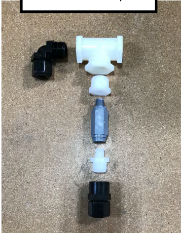
Assembly #2 Flush Tank Input
