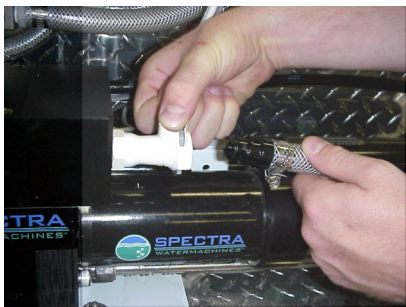
Connecting brine discharge service hose
