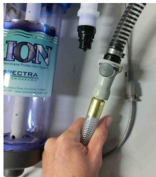
Removing hose to sea strainer from the "to strainer" pigtail.
