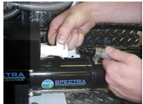
Connecting brine discharge service hose:
